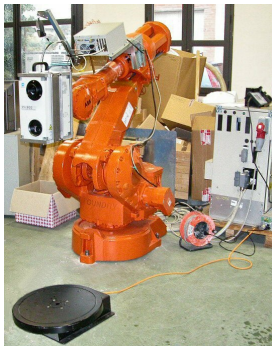
Example of robotized 3D scan setup : RoboScan [11]
