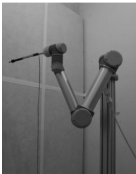
Example of planar robotized acoustic measurements [16]
